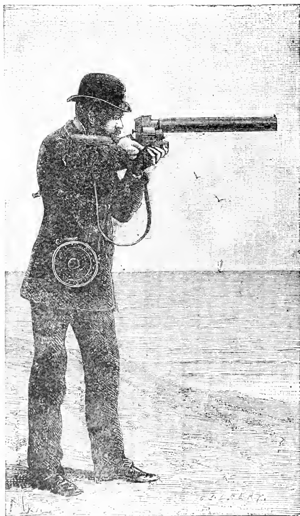
FIG. 17. MODE OF USING THE PHOTOGRAPHIC GUN.
